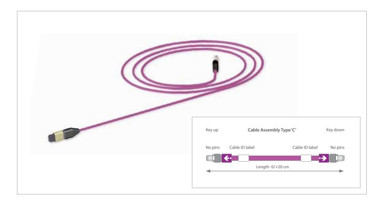
Cable assemblies are made up of 12 fibre LSZH jacketed cables terminated at both ends in MTP® Low Loss connectors (without pins). They are used as backbone or horizontal cable interconnections between distribution racks.
