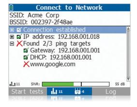
View the process steps on the display and store them in a log for troubleshooting. Quickly test performance and quality of the connection by using the continuous ping response, loss-rate, and connection-range features.
