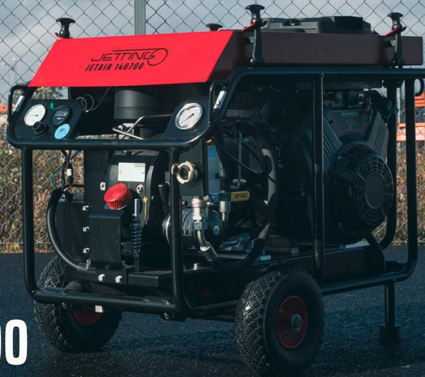
Compact and effective asymmetrical screw-type compressor with aftercooler, optimized for professional fiber blowing.
