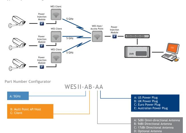
WESII units are supplied with a mid-span compliant power injection module, a 12Vdc 100mA power supply, plus assembly & mounting kit.
