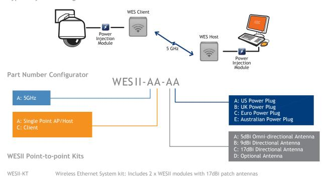
Wireless Ethernet System kit: Includes 2 x WESII modules with 17dBi patch antennas, encoder and decoder
