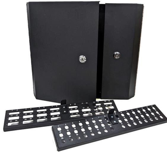
The wall boxes can be supplied with SC duplex, LC quad, ST or FC style adapters. They can be configured for Singlemode or Multimode applications and are available fully loaded, partially loaded or unloaded as required. They are supplied complete with 1 x PG11 gland and 4 x Kurly Loks for cable management.
