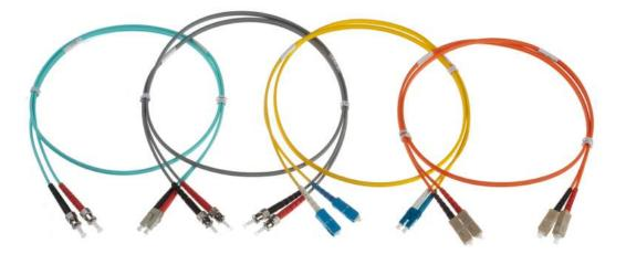
As standard, patch cords are supplied manufactured on 2.8mm diameter cables, with 1.8mm diameter available on request. Cable configurations are simplex, duplex zip cord and duplex flat twin. Multimode patch cords use red and black connector boots and Singlemode patch cords use blue and white connector boots for ease of identification.
