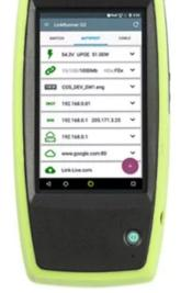
When customization of the AutoTest is needed, profiles can be defined to ensure a standardized test process is executed when variables about the link under test are needed. While these settings can be easily changed in use, profiles can be configured by a senior team member to ensure lessskilled technicians are executing an AutoTest that is specific to their network environment, which is particularly useful in organizations who manage distributed locations.
