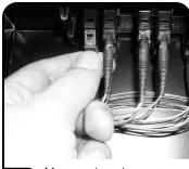
Mate terminated connectors to appropriate ports on the Quick-Pack' adapter plate.
