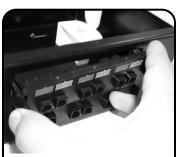
Snap adapter plates into place. Orient the wide edge of the adapter plates to face up as shown. Align the adapter plate latches with the respective cutouts in the mounting bracket and push adapter plate inward until it snaps into place.
