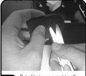
Cut slits in grommet to allow cable to pass through.
