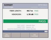
PASS/FAIL insertion loss analysis makes it easy to see whether the fiber is good – and presents the data in a clear, easy-tointerpret format.
