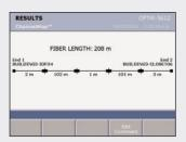
Troubleshooting starts here. See a diagram of the channel, including patch cords. Check that the link is patched all the way across the campus, and identify how many connectors are in a link.
